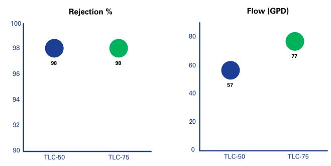
Product Tested at 65 psi; 77°F; 20% recovery; 500 ppm NaCl/RO
