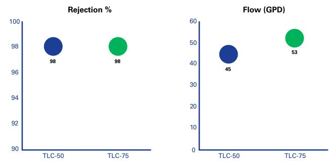
Product Tested at 65 psi; 77°F; 20% recovery; 2000 ppm NaCl/RO
